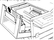
**3** Gently close the printer cover, pressing firmly on both sides of the printer cover until you hear it click.
